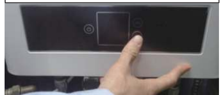
3.2 Quickly long-tap the down icon when you hear "di" and see model code
