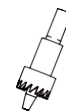
Hole Saws Mode 1: \Phi 24mm Bottom hole (for the single phase) Mode 2: \Phi 18mm (Back hole for Sealing rubber)
